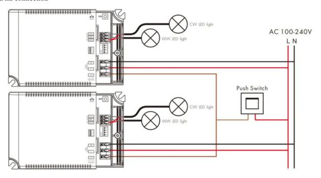
The provided AC Push-Dim interface allows for a simple dimming method using commercially available non-latching (momentary) wall switches.
