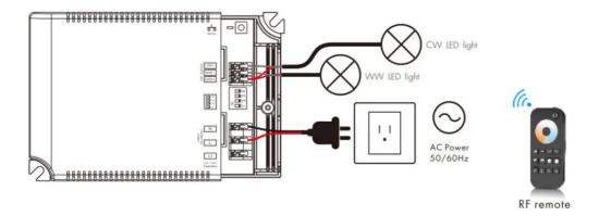
**Note:** Continuously switch off and on the power supply two times rapidly, It will change 3 levels of color temperature (WW, NW, and CW) in sequence.
