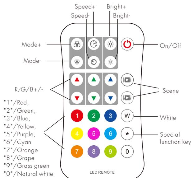
**Mode+/-:** Short press switch dynamic mode built in controller, long press 2s Mode+ run mode cycle, long press 2s Mode- run the first mode. The remote is default 10 dynamic mode, when match with SPI controller which have 32 dynamic mode, please long press 2s Mode+ key firstly.
