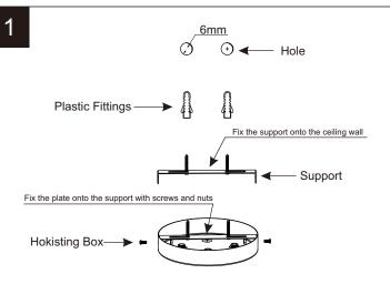
Fixed the box: Firstly, make two 6mm holes on the ceiling wall, then put the into the holes, fixed the support and the box with screws.
