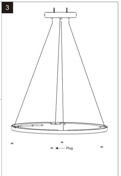
Fixed the light: Press the plate's 4 column one by one, make the iron cord through the column to fix the iron cord, then plug the mounting holes.
