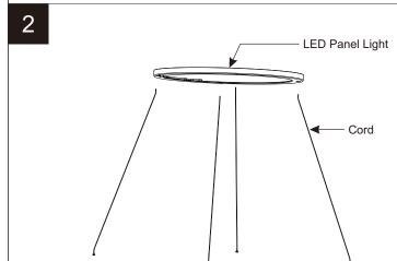
Fixed cord: make the cord through the light's 4 mounting holes.
