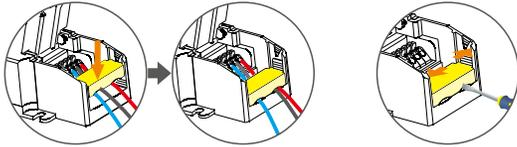
Push the wire pressing board to fix the wire.
