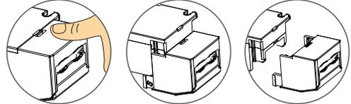
Break off the bottom left and right to remove the protective cover.
