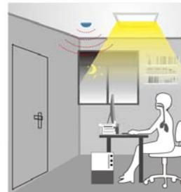
■ It keeps the light on even if the person is stationary for a long time, because it is maintained by breathing detection.
