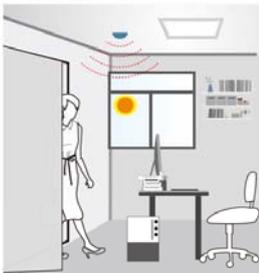
■ When the ambient light is sufficient, the light will not turn on even if the moving signal is detected.
