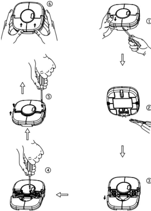
1. Open the corresponding position of the wiring cover by a screw.
