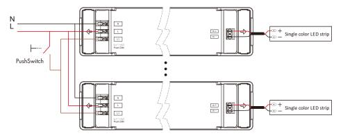
The provided AC Push-Dim interface allows for a simple dimming method using commercially available non-latching (momentary) wall switchs.
