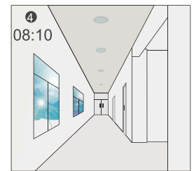
When the natural light level exceeds setpoint off to light, the light will turn off even if when the space is occupied.
